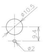
Recommend Installation panel thickness: 2~6mm
